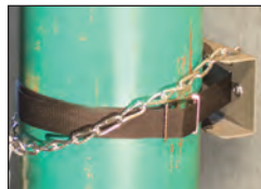
Secure gas cylinders to wall or bench to prevent dangerous tipping.
