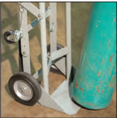
Transport a compressed gas cylinder safely with durable hand truck featuring four wheels for easier, stable transport.
