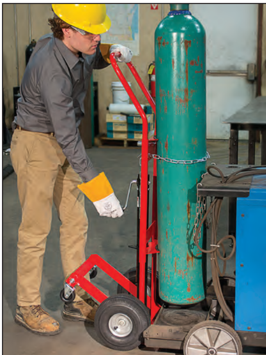
Lift-and-Load hand truck allows user to install heavy cylinders onto raised locations.
